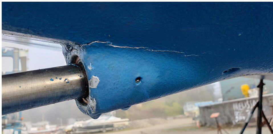
Crack in shaft housing.
