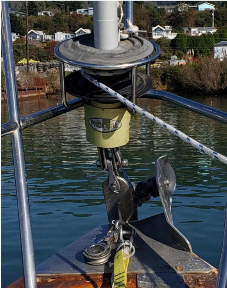
Damage to furler caused by USCG collision.
