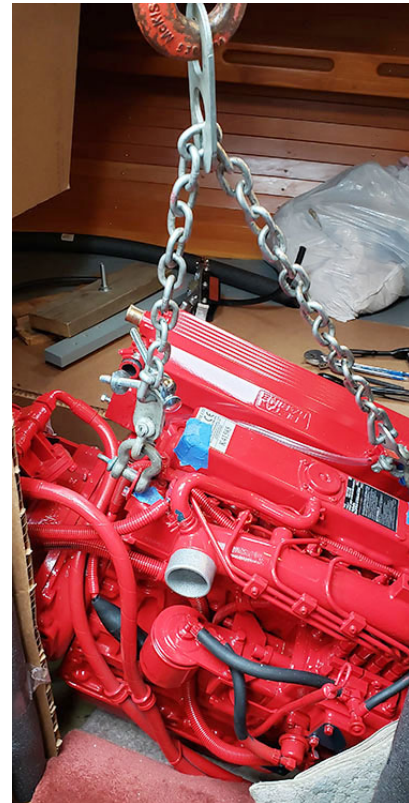
New engine hanging in aft berth
