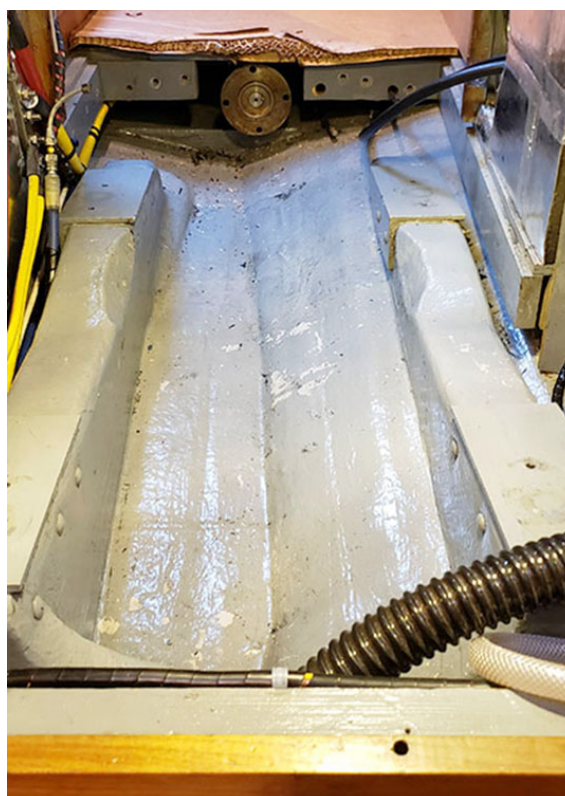
Engine bed, ready for new engine
