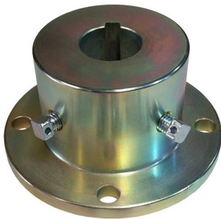
Figure 1. Solid transmission shaft coupling. Note the keyway and the two locking screws which should bear on depressions in the shaft and be seized with wire.
