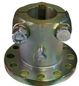
Figure 2. Split transmission coupling. Ideally, both pinch bolt nuts and the setscrew should be drilled for seizing wire.
