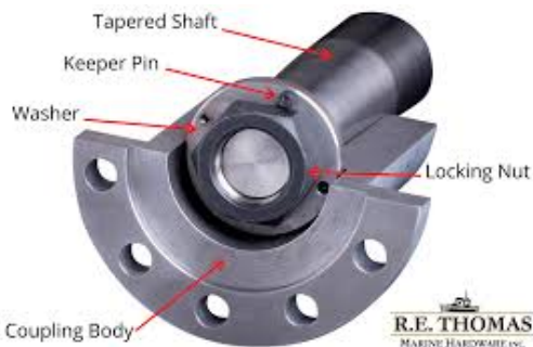
Figure 3: Cutaway view of a tapered shaft coupling. The locking nut and washer provide positive retention when backing down pulls on the shaft.
