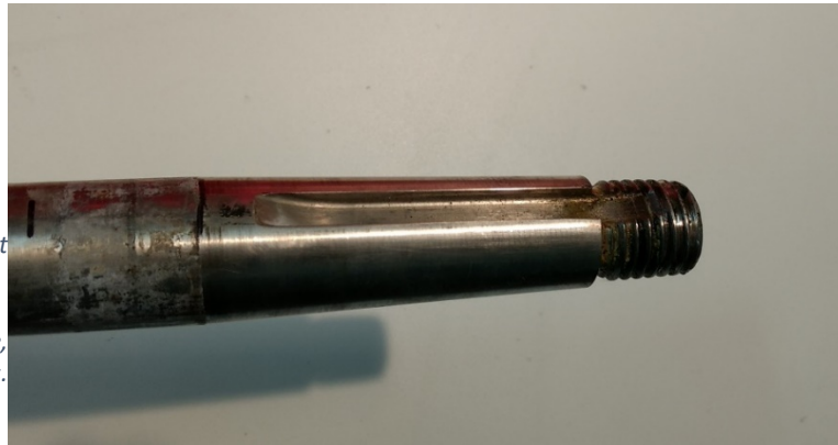
Figure 5. Prop end of shaft. Note that the threaded end is smaller diameter than the body of the shaft. These threads are right-handed, but beware, some shafts have left-handed threads.
