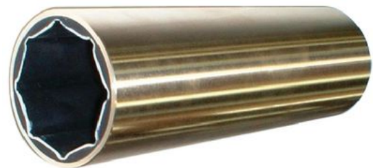
Figure 4. Cutless bearing. This is pressed into a strut or the back of the keel and held in place with setscrews.
