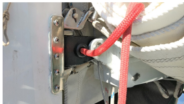
After new riv-nuts and 5200. The red line is for the 3 rd reef tack, which can be pulled down from the cockpit.
